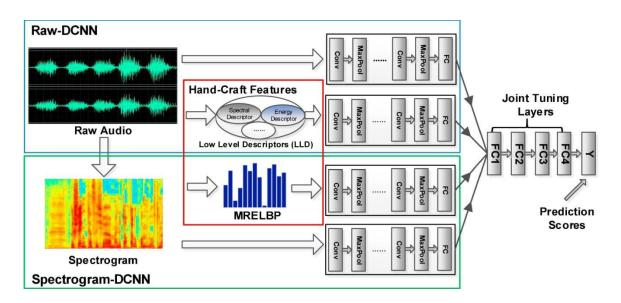
The above figure is the framework for automatic Depression recognition, where Raw-DCNN (Top) takes raw audio signals and low level descriptors (LLD) as input, while the Spectrogram-DCNN (Bottom) uses texture features as input. The red box in above figure is Hand-Crafted features. Other two arrows are Deep-Learned features. The predicted depression score is computed by aggregating or averaging the individual predictions per frame from four DCNNs.
